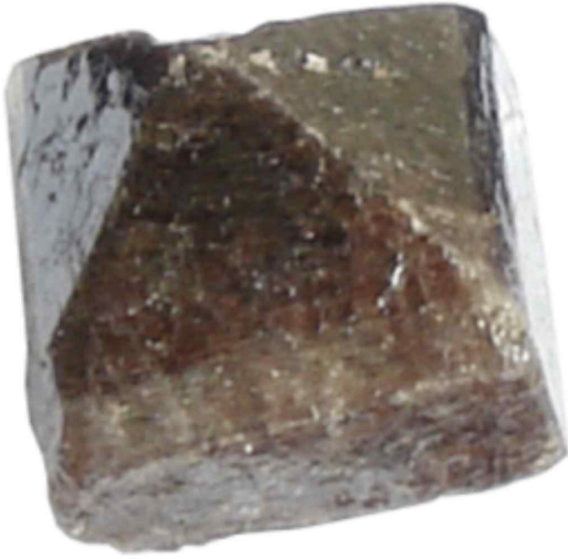
Figure 5-12 Zircon abrasive particle
