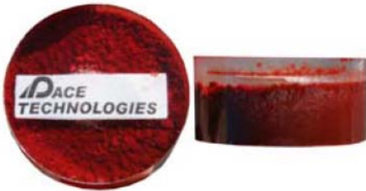
Figure 4-15. Example of labeling mounts using acrylic resin on top of a phenolic base.
