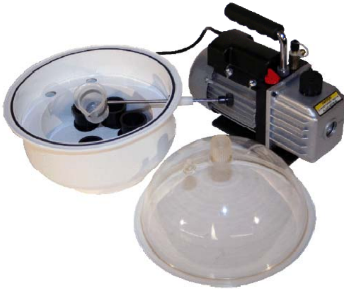
Figure 4-5 Vacuum impregnation device.
