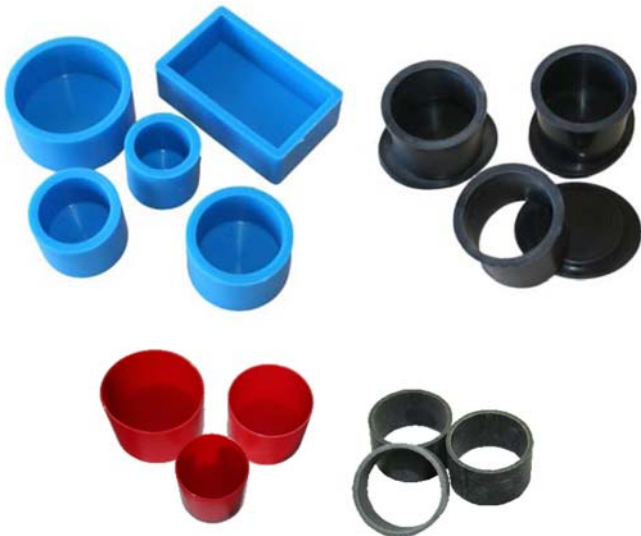
Figure 4-6 Cold mounting molds(clockwise: silicon rubber, 2-piece plastic, ring forms, disposable).
