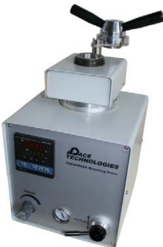
Figure 4-10 Compression Mounting Press.
