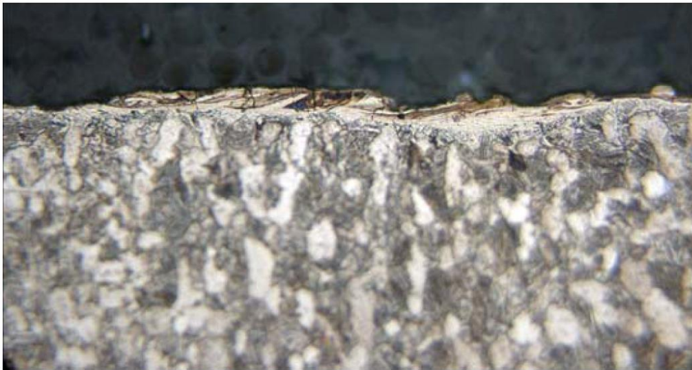
Figure 6-19 Edge rounding at edge of titanium and mount.
