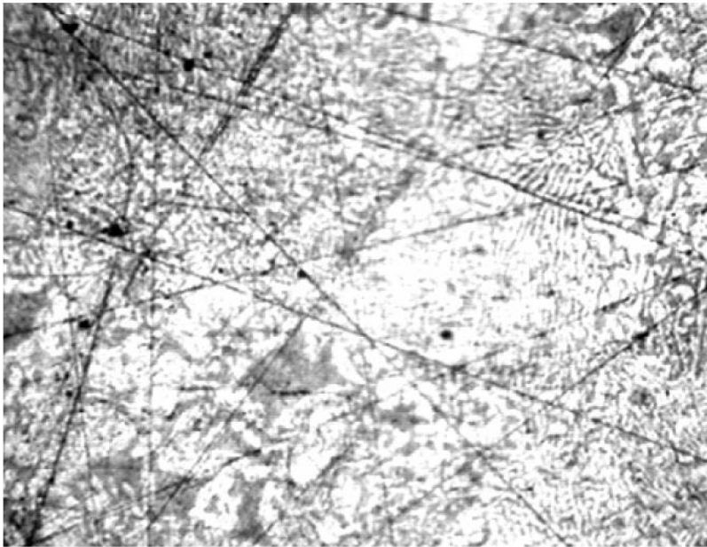
Figure 6-14a Bismuth-tin alloy prior to polish-etch-polish.
