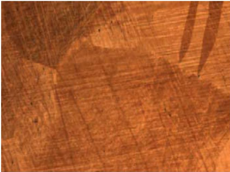
Figure 6-12b Tin after attack polishing with 2% Nital, mag. 50X.
