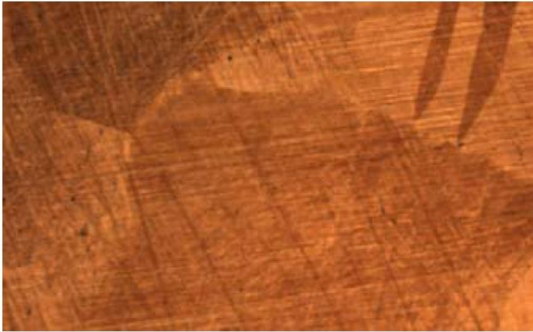
Figure 6-16b Large tin grains following attack polishing with 2% Nital.
